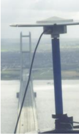
Figure 8 - The Ashtech ZXII Antenna Located on top of the Support Tower
